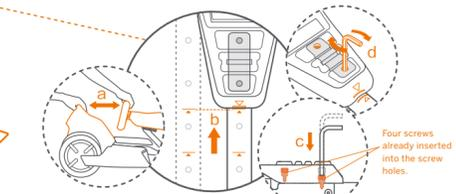
⑧ Stretch the frame and adjust the length of the body:
