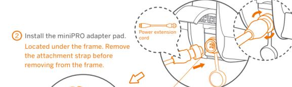
② Install the miniPRO adapter pad. Located under the frame. Remove the attachment strap before removing from the frame.
